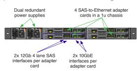
With 80 Gb throughput, a single chassis can comfortably support simultaneous access to 80 drives w/ equivalent performance to direct attached storage
