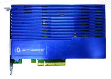
Infused with the BiTMICRO® Talino™ architecture, MAXio Z-Series PCle SSDs include two in-house developed ASIC flash controllers for enhanced application performance. Offloading the Flash Translation Layer (FTL) from the host server to the SSD, MAXio Z-Series PCle SSDs support higher storage capacities up to 8.8 TB in a PCle edge card form factor. DriveLight™ Management Software allows users to simplify MAXio SSD administration with easy-to-use, interactive features.
